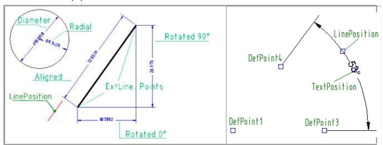
Angular dimensions measure the angle between two lines or three points.
