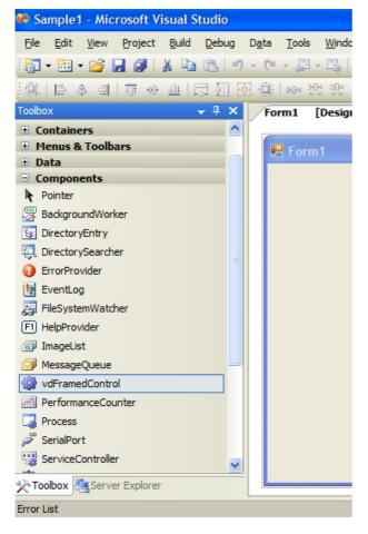
6) Add it to the form and also 4 buttons that will do some simple functions like Open/Save a drawing. Create a new drawing and Zoom Extends.
